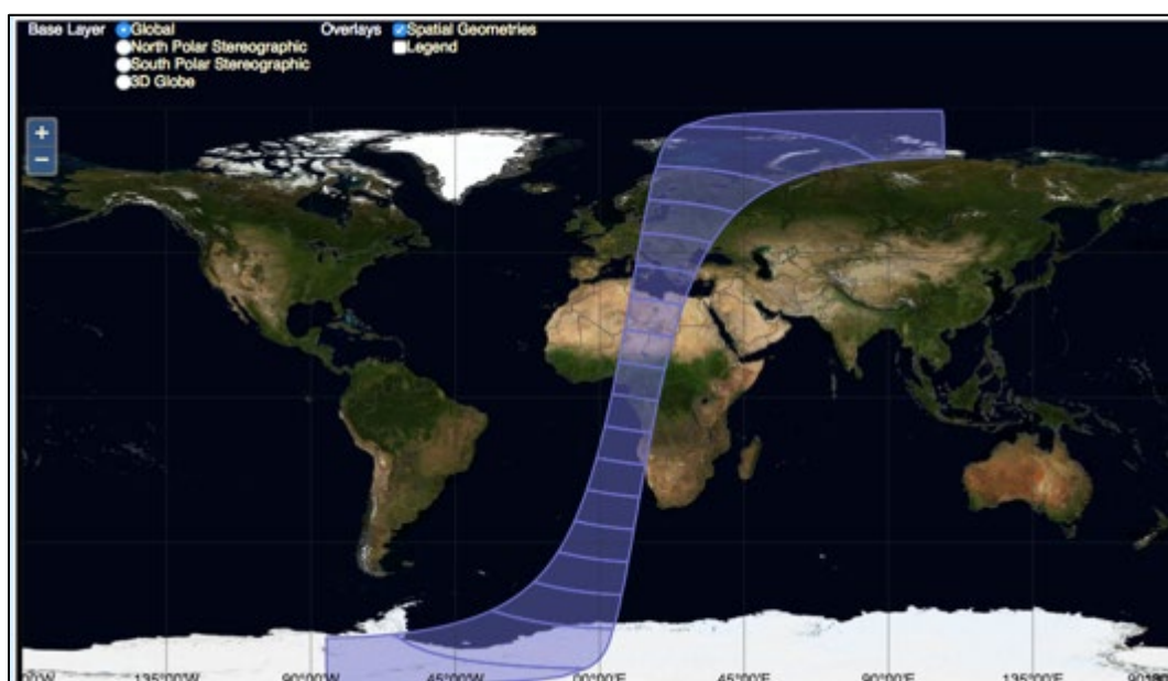
Figure 2. Swath coverage during one half orbit of the AMSR-E instrument.
