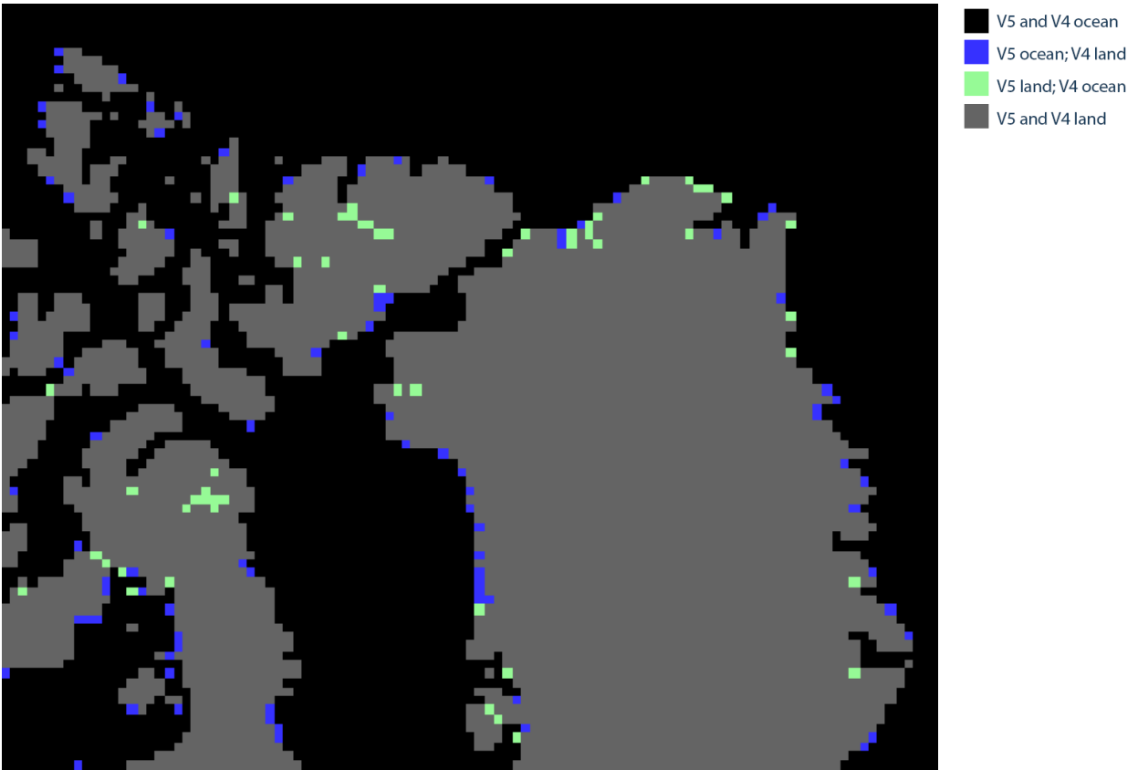
Figure 6. Cropped area showing the differences between the V4 and V5 land mask around the Canadian Arctic Archipelago and Greenland. Black: Both V4 and V5 agree a grid cell is ocean. Blue: V5 indicates a grid cell is ocean, whereas V4 had it as land. Green: V5 indicates a grid cell is land, whereas V4 had it as ocean. Gray: Both V4 and V5 agree a grid cell is land (i.e. land, lake, or coast).
