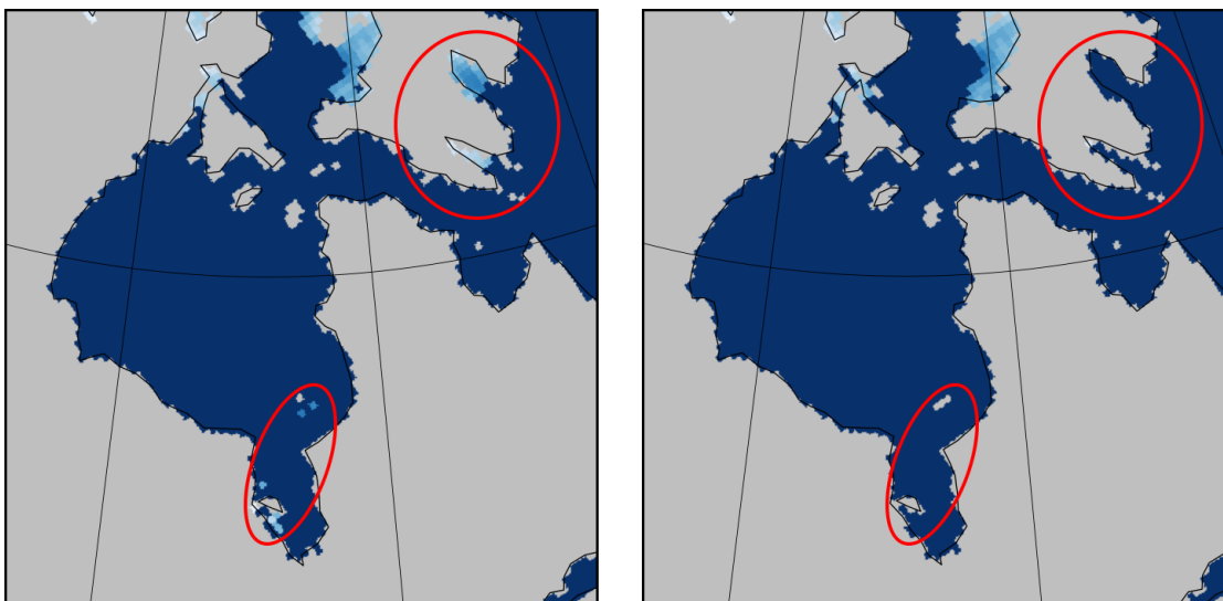
Figure 5. Differences in the effectiveness of NT (left) and NT2 (right) land-spillover corrections for 13 August 2023. The areas circled in red show areas of ice left by the NT algorithm (left) but that are removed by the NT2 algorithm (right).
