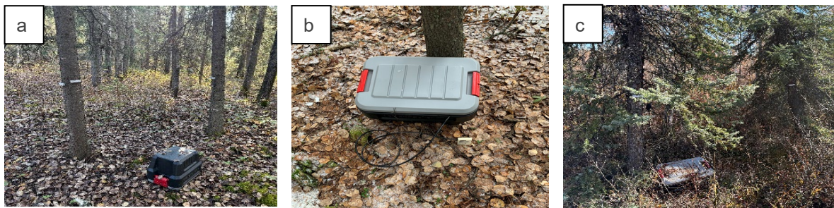
Figure 2. Pictures of TEROS 12 sensors installed into white spruce trees at BCEF1 (a), the CS650 sensor installed at BCEF1 (b), and the TEROS 12 sensors installed into black spruce trees at BCEF2 (c). White arrows are pointing to the location of the sensors.
