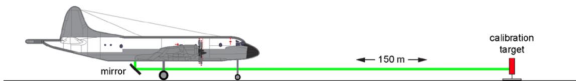
Figure 4. Range bias determination (a.k.a. ground test) using a calibration target with a known distance. The distance to the calibration target is measured with an electronic distance meter (a.k.a. total station) with an accuracy of a few millimeters.
